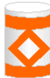
Figure 1-5a: An example of a buoy used to mark a boating hazard. The buoy is conventionally white with red or orange diamond and stripes
